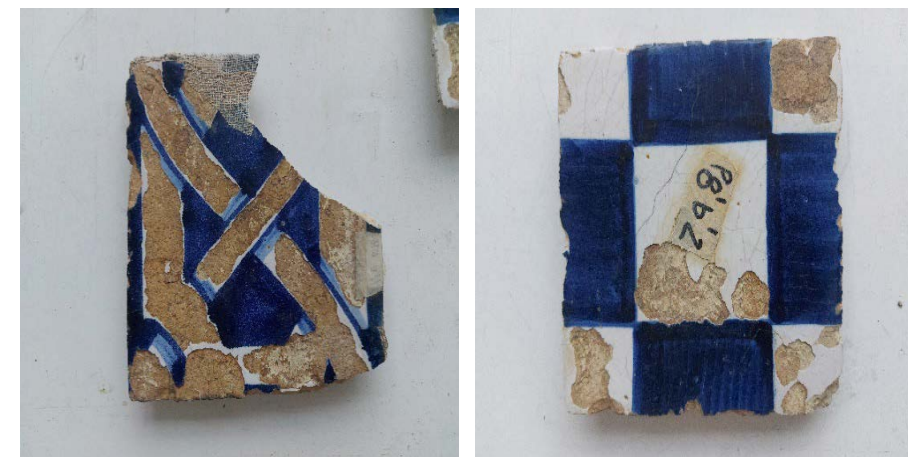
Figure 1 and 2: Examples of glaze detachment specific to the white glaze.
