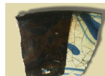
Figure 1. Fragment of blackened Delftware (c. 1660-1680, found in Amsterdam) illustrating recovery of the original glaze design in the right-hand portion which was exposed to Lisbon summer sun for 12 weeks.
