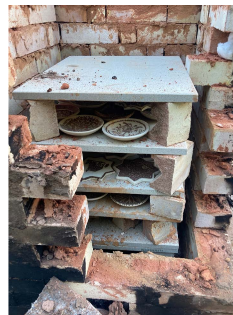
Figure 2. The lustre-firing kiln we reconstructed as part of our replication experiment at the Fitzwilliam Museum, University of Cambridge (photo taken by Carmen Ting).
