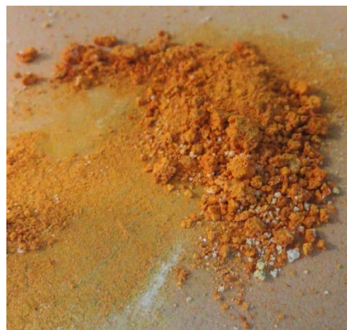
Figure 2. Laboratory replication of a Naples Yellow historical pigment recipe
